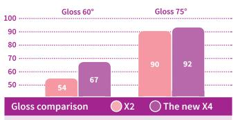
Gloss comparison between Extrachrome X2 and Extrachrome X4 grade. Typical value for Gloss 60° is over 65 GU (gloss unit). Measurement method is based on ISO 2813 standard.
